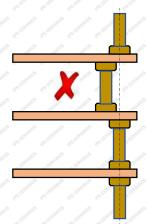
The same principle applies when building up the kiln car, ie. Each level relies on the components immediately below, and so it's essential that the props used to support each deck are aligned directly above the supports below. This allows the weight to transfer down into the car base.
