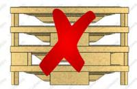
For deeper setters, the depth of the setter can be greater than the spacer height, so that the spacer does not reach the support below. In this case a few setters should be cemented using taller spacers (for use as a base setter) or a support ring can also be used.
