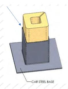
The bolted socket provides a tighter fit to the post, but it is important that the posts are still able to move slightly, as this helps the overall stability of the kiln car structure. **The bolts should be finger tightened only**; over tightening will result in breakage of the post as the kiln car is moved – which may cause a collapse of the structure.
