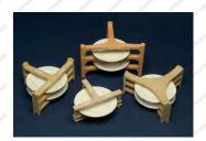
**Total Foot Supports (TFS)** – These are effectively a small batt that gives full support to the foot of a plate during firing, minimising distortion. As with T-Cranks, they are available with or without integral legs.
