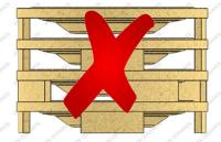
If the depth of the setter is greater than the spacer height, the bottom setter should be lifted using a ring, base setter or taller dots.
