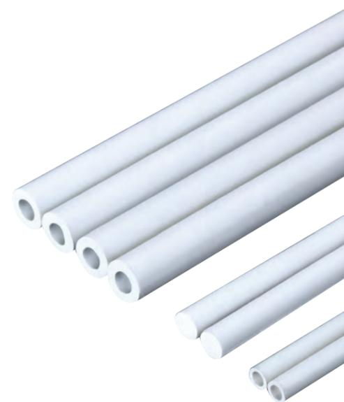
Alumina is the most widely used technical ceramic and is the material of choice in about 80% of engineering applications due to its combination of properties. Fired at over 1600°C (2900°F) to give a fully dense technical ceramic, alumina exhibits high mechanical strength, rigidity and can be machined to tight tolerances and fine surface finishes. Alumina is often used as a replacement for metallic components in demanding engineering applications.
