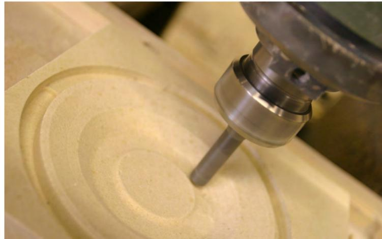
IPS Ceramics manufactures a low density, porous, cordierite material that can be easily machined.
