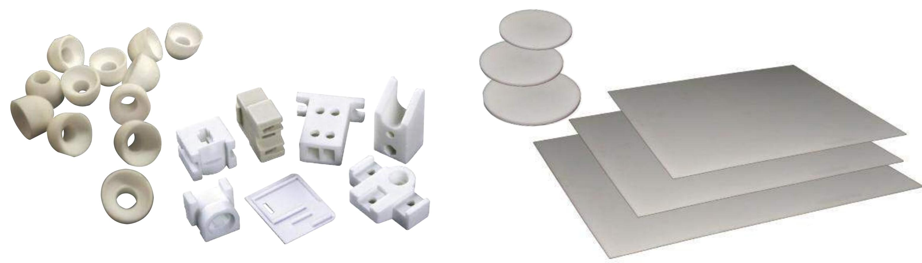
**Steatite** is used extensively in the electrical and electronic industries. High grade steatite ceramics are low-loss materials which exhibit excellent dielectric and mechanical properties. Wherever good electrical insulation is required, including high voltages and at elevated temperatures (up to 1200°C/2200°F) then steatite should be considered.
