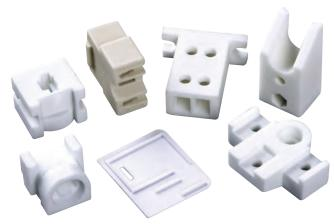
Steatite is used extensively for insulation in the electrical and electronic industries. It is a lower cost material than alumina, but has excellent electrical resistance properties (which are retained at high temperatures) along with moderate mechanical strength.
