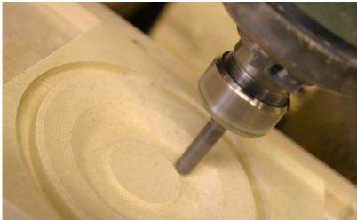
IPS Ceramics manufactures a low density, porous, cordierite material that can be easily machined.
