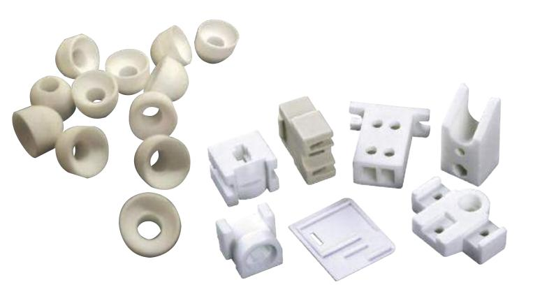
Steatite is used extensively in the electrical and electronic industries. High grade steatite ceramics are low-loss materials which exhibit excellent dielectric and mechanical properties. Wherever good electrical insulation is required, including high voltages and at elevated temperatures (up to 1200°C/2200°F) then steatite should be considered.
